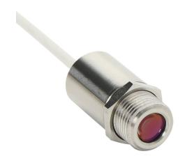
Optris CSmicro 2M infrared pyrometer, 385 to 1600 deg C, 1.6  $\mu$ m spectral range, 0-5 VDC, 0-10 VDC, alarm or pulse output, 5-30 VDC operating voltage, M12x1 threaded end mount, 6m integral 5-conductor shielded cable.
