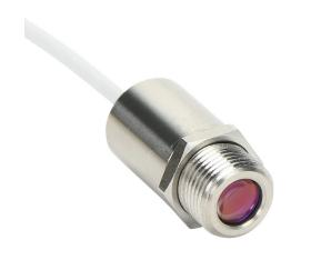
Optris CSmicro 2M infrared pyrometer, 385 to 1600 deg C, 1.6  $\mu$ m spectral range, 0-5 VDC, 0-10 VDC, alarm or pulse output, 5-30 VDC operating voltage, M12x1 threaded end mount, 1m integral 5-conductor shielded cable.
