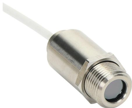
Optris CSmicro LTH infrared pyrometer, -50 to 1030 deg C, 8-14  $\mu\text{m}$  spectral range, 4-20 mA, alarm or pulse output, 5-30 VDC operating voltage, M12x1 threaded end mount, 6m integral 5-conductor shielded cable.
