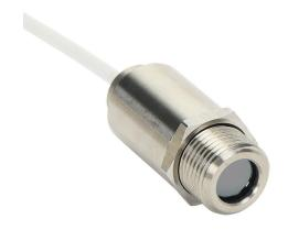
Optris CSmicro LTH infrared pyrometer, -50 to 1030 deg C, 8-14  $\mu$ m spectral range, 4-20 mA, alarm or pulse output, 5-30 VDC operating voltage, M12x1 threaded end mount, 6m integral 5-conductor shielded cable.
