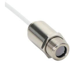
Optris CSmicro LTH infrared pyrometer, -50 to 1030 deg C, 8-14  $\mu$ m spectral range, 4-20 mA, alarm or pulse output, 5-30 VDC operating voltage, M12x1 threaded end mount, 1m integral 5-conductor shielded cable.
