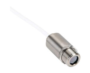
Optris CSmicro LT infrared pyrometer, -50 to 1030 deg C, 8-14 µm spectral range, 4-20 mA, alarm or pulse output, 5-30 VDC operating voltage, M12x1 threaded end mount, 6m integral 5-conductor shielded cable.
