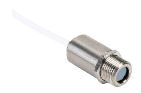
Optris CSmicro LT infrared pyrometer, -50 to 1030 deg C, 8-14  $\mu$ m spectral range, 4-20 mA, alarm or pulse output, 5-30 VDC operating voltage, M12x1 threaded end mount, 1m integral 5-conductor shielded cable.
