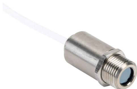
Optris CSmicro LT infrared pyrometer, -50 to 1030 deg C, 8-14  $\mu\text{m}$  spectral range, 4-20 mA, alarm or pulse output, 5-30 VDC operating voltage, M12x1 threaded end mount, 1m integral 5-conductor shielded cable.
