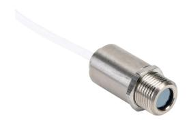
Optris CSmicro LT infrared pyrometer, -50 to 1030 deg C, 8-14  $\mu$ m spectral range, 4-20mA, alarm or pulse output, 5-30 VDC operating voltage, M12x1 threaded end mount, 1m integral 5-conductor shielded cable.
