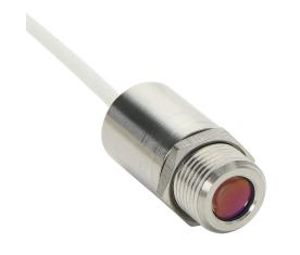
Optris CSmicro 3M infrared pyrometer, 50 to 350 deg C, 2.3  $\mu$ m spectral range, 4-20 mA, alarm or pulse output, 5-30 VDC operating voltage, M12x1 threaded end mount, 6m integral 5-conductor shielded cable.
