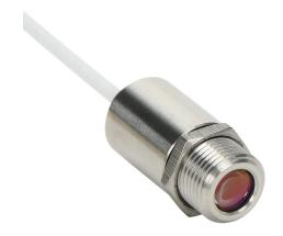
Optris CSmicro 3M infrared pyrometer, 50 to 350 deg C, 2.3  $\mu$ m spectral range, 4-20 mA, alarm or pulse output, 5-30 VDC operating voltage, M12x1 threaded end mount, 1m integral 5-conductor shielded cable.
