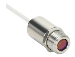
Optris CSmicro 3M infrared pyrometer, 100 to 600 deg C, 2.3  $\mu$ m spectral range, 4-20 mA, alarm or pulse output, 5-30 VDC operating voltage, M12x1 threaded end mount, 6m integral 5-conductor shielded cable.
