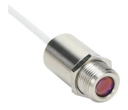
Optris CSmicro 3M infrared pyrometer, 100 to 600 deg C, 2.3  $\mu$ m spectral range, 4-20 mA, alarm or pulse output, 5-30 VDC operating voltage, M12x1 threaded end mount, 1m integral 5-conductor shielded cable.
