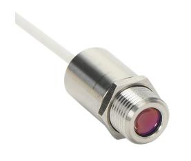
Optris CSmicro 2M infrared pyrometer, 385 to 1600 deg C, 1.6  $\mu$ m spectral range, 4-20 mA, alarm or pulse output, 5-30 VDC operating voltage, M12x1 threaded end mount, 6m integral 5-conductor shielded cable.
