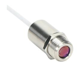
Optris CSmicro 2M infrared pyrometer, 385 to 1600 deg C, 1.6  $\mu$ m spectral range, 4-20 mA, alarm or pulse output, 5-30 VDC operating voltage, M12x1 threaded end mount, 1m integral 5-conductor shielded cable.
