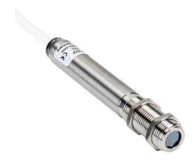
Optris CS LT infrared pyrometer, -50 to 1030 deg C, 8-14  $\mu$ m spectral range, 0-5 VDC, 0-10 VDC, Type K thermocouple, alarm or pulse output, 5-30 VDC operating voltage, M12x1 threaded end mount, 8m integral 7-conductor shielded cable.
