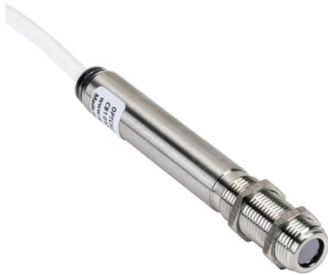
Optris CS LT infrared pyrometer, -50 to 1030 deg C, 8-14  $\mu\text{m}$  spectral range, 0-5 VDC, 0-10 VDC, Type K thermocouple, alarm or pulse output, 5-30 VDC operating voltage, M12x1 threaded end mount, 1m integral 7-conductor shielded cable.
