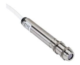
Optris CS LT infrared pyrometer, -50 to 1030 deg C, 8-14 µm spectral range, 0-5 VDC, 0-10 VDC, Type K thermocouple, alarm or pulse output, 5-30 VDC operating voltage, M12x1 threaded end mount, 1m integral 7-conductor shielded cable.
