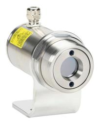
Optris CSlaser LT infrared pyrometer, -30 to 1000 deg C, 8-14  $\mu$ m spectral range, 4-20 mA and alarm output, 5-30 VDC operating voltage, M48x1.5 threaded end mount, removable screw terminal plug.
