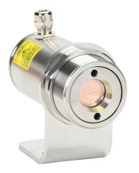
Optris CSlaser 2M infrared pyrometer, 250 to 800 deg C, 1.6  $\mu$ m spectral range, 4-20 mA and alarm output, 5-30 VDC operating voltage, M48x1.5 threaded end mount, removable screw terminal plug.
