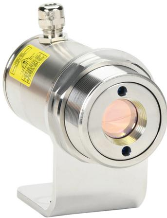
Optris CSLaser 2M infrared pyrometer, 250 to 800 deg C, 1.6  $\mu\text{m}$  spectral range, 4-20 mA and alarm output, 5-30 VDC operating voltage, M48x1.5 threaded end mount, removable screw terminal plug.
