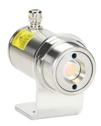
Optris CSlaser 2M infrared pyrometer, 385 to 1600 deg C, 1.6  $\mu$ m spectral range, 4-20 mA and alarm output, 5-30 VDC operating voltage, M48x1.5 threaded end mount, removable screw terminal plug.
