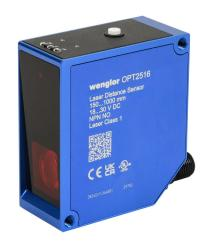
Wenglor photoelectric sensor, rectangular, diffuse, Class 1 red laser, 150-1000mm sensing distance, (2) NPN, teach-in button, 650 Hz switching frequency, aluminum housing, 5-pin M12 quick-disconnect.
