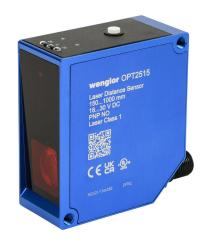
Wenglor photoelectric sensor, rectangular, diffuse, Class 1 red laser, 150-1000mm sensing distance, (2) PNP, teach-in button, 650 Hz switching frequency, aluminum housing, 5-pin M12 quick-disconnect.
