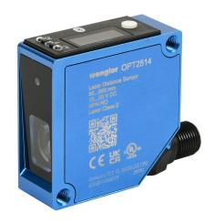
Wenglor photoelectric sensor, square, diffuse, Class 2 blue laser, 60-660mm sensing distance, (2) NPN, teach-in button, 650 Hz switching frequency, aluminum housing, 5-pin M12 quick-disconnect.
