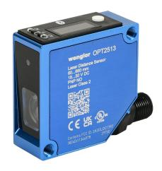
Wenglor photoelectric sensor, square, diffuse, Class 2 blue laser, 60-660mm sensing distance, (2) PNP, teach-in button, 650 Hz switching frequency, aluminum housing, 5-pin M12 quick-disconnect.
