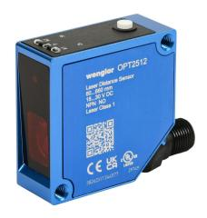
Wenglor photoelectric sensor, square, diffuse, Class 1 red laser, 60-660mm sensing distance, (2) NPN, teach-in button, 650 Hz switching frequency, aluminum housing, 5-pin M12 quick-disconnect.
