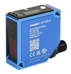
Wenglor photoelectric sensor, square, diffuse, Class 1 red laser, 60-660mm sensing distance, teach-in button, aluminum housing, 5-pin M12 quick-disconnect.
