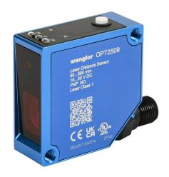
Wenglor photoelectric sensor, square, diffuse, Class 1 red laser, 60-660mm sensing distance, (2) PNP, teach-in button, 650 Hz switching frequency, aluminum housing, 5-pin M12 quick-disconnect.
