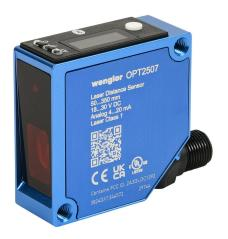
Wenglor photoelectric sensor, square, diffuse, Class 1 red laser, 50-350mm sensing distance, teach-in button, aluminum housing, 5-pin M12 quick-disconnect.
