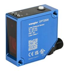
Wenglor photoelectric sensor, square, diffuse, Class 1 red laser, 50-350mm sensing distance, (2) PNP, teach-in button, 650 Hz switching frequency, aluminum housing, 5-pin M12 quick-disconnect.
