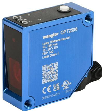
Wenglor photoelectric sensor, square, diffuse, Class 1 red laser, 50-350mm sensing distance, (2) PNP, teach-in button, 650 Hz switching frequency, aluminum housing, 5-pin M12 quick-disconnect.
