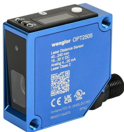
Wenglor photoelectric sensor, square, diffuse, Class 2 blue laser, 40-240mm sensing distance, teach-in button, aluminum housing, 5-pin M12 quick-disconnect.
