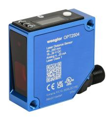
Wenglor photoelectric sensor, square, diffuse, Class 1 red laser, 40-240mm sensing distance, teach-in button, aluminum housing, 5-pin M12 quick-disconnect.
