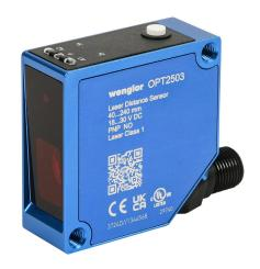
Wenglor photoelectric sensor, square, diffuse, Class 1 red laser, 40-240mm sensing distance, (2) PNP, teach-in button, 650 Hz switching frequency, aluminum housing, 5-pin M12 quick-disconnect.
