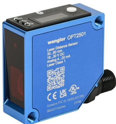
Wenglor photoelectric sensor, square, diffuse, Class 1 red laser, 30-80mm sensing distance, teach-in button, aluminum housing, 5-pin M12 quick-disconnect.
