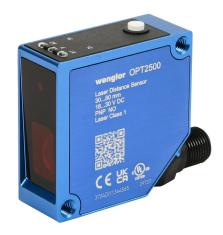
Wenglor photoelectric sensor, square, diffuse, Class 1 red laser, 30-80mm sensing distance, (2) PNP, teach-in button, 650 Hz switching frequency, aluminum housing, 5-pin M12 quick-disconnect.
