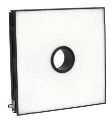
WenglorTPL HPF-DOME machine vision lighting, flat dome light, infrared light emission,  $300 \times 300$ mm luminous field,  $320 \times 320 \times 45$ mm housing, 24 VDC operating voltage.
