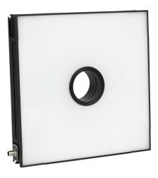
WenglorTPL HPF-DOME machine vision lighting, flat dome light, white light emission, 5700K, 300 x 300mm luminous field, continuous and strobe, 320 x 320 x 45mm housing, 24 VDC operating voltage.
