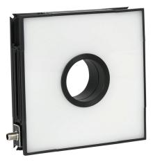
WenglorTPL HPF-DOME machine vision lighting, flat dome light, infrared light emission, 200 x 200mm luminous field, continuous and strobe, 220 x 220 x 45mm housing, 24 VDC operating voltage.
