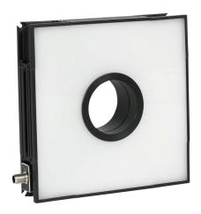
WenglorTPL HPF-DOME machine vision lighting, flat dome light, infrared light emission,  $200 \times 200 \text{mm}$  luminous field,  $220 \times 220 \times 45 \text{mm}$  housing, 24 VDC operating voltage.
