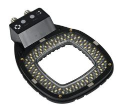
WenglorTPL Modular-RING 80mm machine vision lighting, ring light, white and infrared light emission, 5000K, plus or minus 65 degrees, continuous and strobe, 136 x 181 x 31mm housing, 21.6-30 VDC operating voltage.
