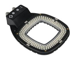
WenglorTPL Modular-RING 80mm machine vision lighting, ring light, visible red and cyan light emission, plus or minus 65 degrees, continuous and strobe, 136 x 181 x 31mm housing, 21.6-30 VDC operating voltage.
