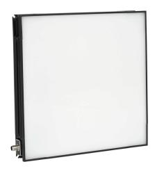
WenglorTPL HP-BACK machine vision lighting, backlight, infrared light emission, 300 x 300mm luminous field, 320 x 320 x 45mm housing, 24 VDC operating voltage.
