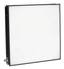
WenglorTPL HP-BACK machine vision lighting, backlight, white light emission, 5700K,  $300 \times 300$ mm luminous field,  $320 \times 320 \times 45$ mm housing, 24 VDC operating voltage.
