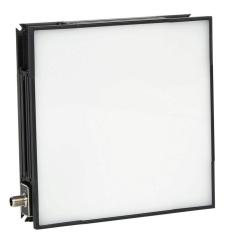
WenglorTPL HP-BACK machine vision lighting, backlight, infrared light emission, 200 x 200mm luminous field, continuous and strobe, 220 x 220 x 45mm housing, 24 VDC operating voltage.
