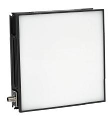
WenglorTPL HP-BACK machine vision lighting, backlight, white light emission, 5700K, 200 x 200mm luminous field, continuous and strobe,  $220 \times 220 \times 45$ mm housing, 24 VDC operating voltage.
