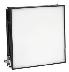
WenglorTPL HP-BACK machine vision lighting, backlight, white light emission, 5700K,  $200 \times 200$ mm luminous field,  $220 \times 220 \times 45$ mm housing, 24 VDC operating voltage.
