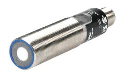
Wenglor ultrasonic proximity sensor, tubular, 18mm diameter x 86mm body, stainless steel housing, PNP, 0-10 VDC analog output, N.O., 50-400mm sensing distance, 20 Hz switching frequency, IP67, 5-pin M12 quick-disconnect.
