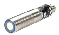
Wenglor ultrasonic proximity sensor, tubular, 18mm diameter x 95mm body, stainless steel housing, PNP, 0-10 VDC analog output, N.O., 100-1200mm sensing distance, 7 Hz switching frequency, IP67, 5-pin M12 quick-disconnect.
