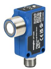
Wenglor ultrasonic proximity sensor, rectangular, 56.5 x 16 x 35mm body, polybutylene terephthalate housing, NPN, N.O., 1-2000mm sensing distance, 7 Hz switching frequency, IP67 IP68, 5-pin M12 quick-disconnect.
