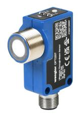
Wenglor ultrasonic proximity sensor, rectangular, 56.5 x 16 x 35mm body, polybutylene terephthalate housing, PNP, N.O., 1-2000mm sensing distance, 7 Hz switching frequency, IP67 IP68, 5-pin M12 quick-disconnect.
