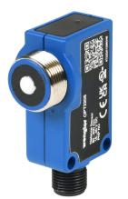
Wenglor ultrasonic proximity sensor, rectangular, 56.5 x 16 x 35mm body, polybutylene terephthalate housing, PNP, N.O., 80-400mm sensing distance, 20 Hz switching frequency, IP67 IP68, 4-pin M12 quick-disconnect.
