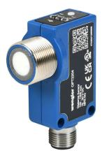
Wenglor ultrasonic proximity sensor, rectangular, 56.5 x 16 x 35mm body, polybutylene terephthalate housing, NPN, N.O., 100-1200mm sensing distance, 7 Hz switching frequency, IP67 IP68, 5-pin M12 quick-disconnect.
