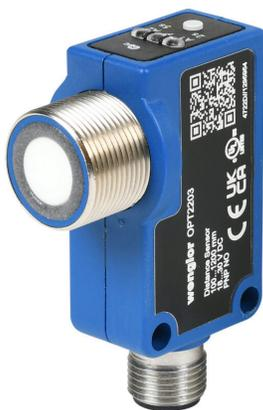
Wenglor ultrasonic proximity sensor, rectangular, 56.5 x 16 x 35mm body, polybutylene terephthalate housing, PNP, N.O., 100-1200mm sensing distance, 7 Hz switching frequency, IP67 IP68, 5-pin M12 quick-disconnect.
