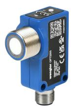
Wenglor ultrasonic proximity sensor, rectangular, 56.5 x 16 x 35mm body, polybutylene terephthalate housing, PNP, N.O., 100-1200mm sensing distance, 7 Hz switching frequency, IP67 IP68, 5-pin M12 quick-disconnect.
