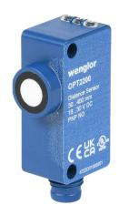
Wenglor ultrasonic proximity sensor, rectangular, 38.5 x 19.5 x 12mm body, polycarbonate housing, PNP, N.O., 30-400mm sensing distance, 30 Hz switching frequency, IP68, 4-pin M8 quick-disconnect.
