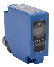
Wenglor photoelectric sensor, square, plastic, diffuse with background suppression, 0-3m sensing distance, complementary light-on/dark-on, NPN, teach-in button, 500 Hz switching frequency, 5-pin M12 quick-disconnect.
