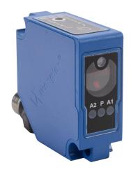
Wenglor photoelectric sensor, square, plastic, diffuse with background suppression, 0-3m sensing distance, complementary light-on/dark-on, PNP, teach-in button, 500 Hz switching frequency, 5-pin M12 quick-disconnect.
